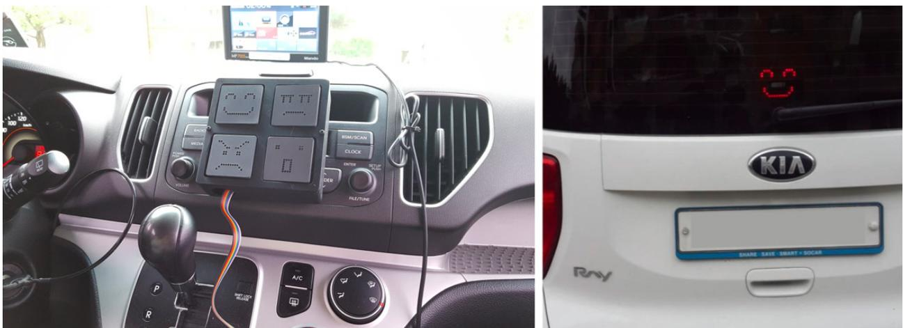
Figure 5. Design artifact: emoticon buttons (left) and LED display on the rear window (right).
