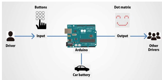
Figure 2. System diagram of the prototype
