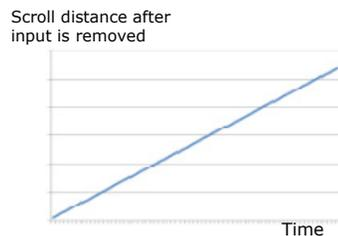
**figure 4.** Scroll behavior with exaggerated inertial effect (coefficient of friction=0.005)
