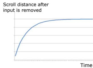
**figure 3.** Scroll behavior with proper inertial effect (coefficient of friction=0.08)
