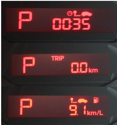
figure 4. KIA Soul trip computer, which indicates the overall driving time (top), driving distance (middle), and average fuel consumption (bottom)
