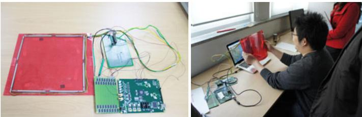
**Fig. 2.** FlexRemote prototype (left) and user study (right)
